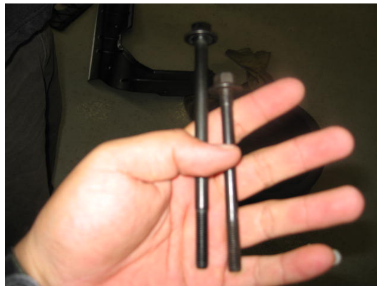
Shorter bolt used on bottom of Condenser
