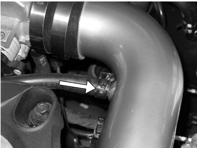
j) Secure the breather hose to the inlet pipe with the original spring clamp
