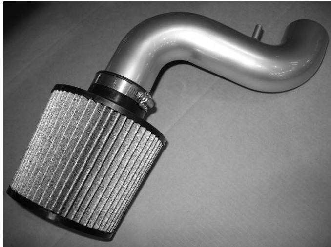
f) Attach the coupler onto the throttle body. Secure it with a size 40 hose clamp.
