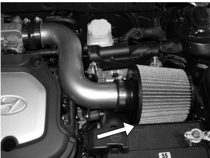
l) Adjust the inlet pipe, vibration mount and heat shield so that no part of the intake is contacting the vehicle. **Be especially mindful of the clearance between the battery and the air filter.** Tighten all bolts, hose clamps and flange nuts
