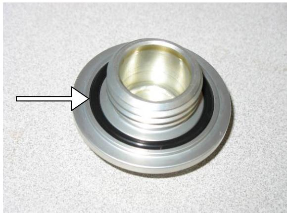
c) Install O ring in oil cap.
