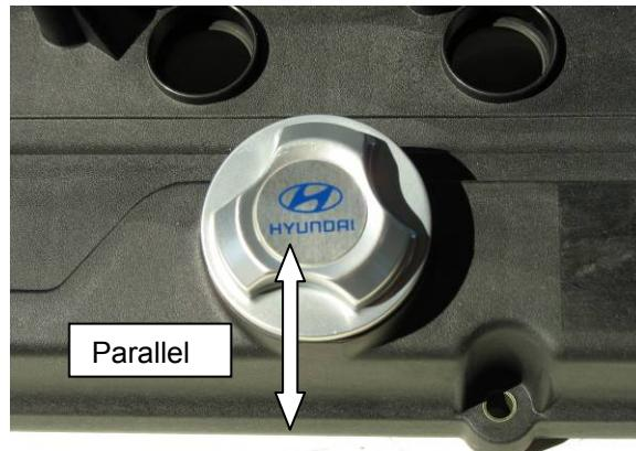
c) Hand tighten the cap. Apply the Hyundai decal after first aligning the text with the front of the valve cover.
