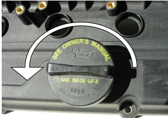
a) Remove the original oil filler cap.
