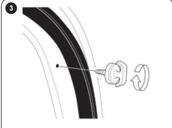
• Use pliers to start screwing in the T-anchor, then hand-tighten in place.
