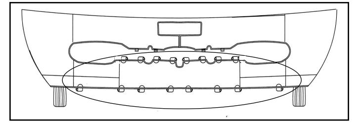
Pre-bend tabs and attach to the edge of the structure.
